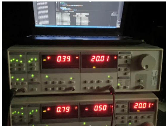
Figure. 16 Lock-in amplifiers; Stanford Research SR810 (top) and SR830 (bottom)
