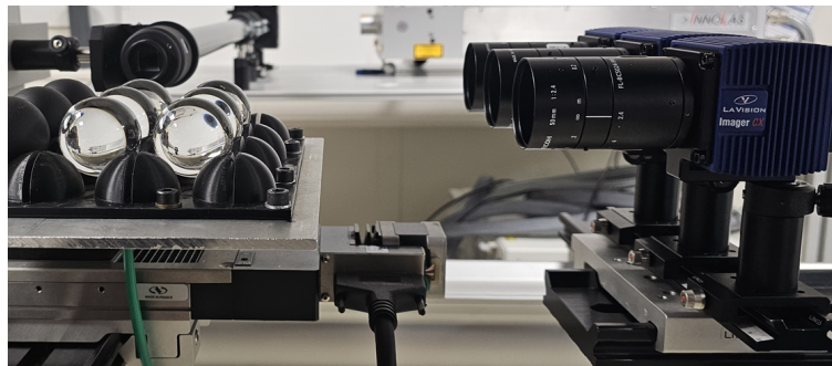
Figure 2 Integration of Configuration 2 in the PIV-Setup. A gas jet ( Re=5900 ) provided by a tube with an inner diameter of d_i=4\text{mm} surrounds the central sphere of a two-layer packed bed of d=40\text{mm} spheres in bcc arrangement. Note that in the real measurements, contrary to the image, the cameras are placed further away to be able to generate the necessary depth of field for performing RT-PIV. The setup allows to use three cameras for the investigation of different perspectives to the measurement plane. For the data presented in this study, only the central camera is used.
