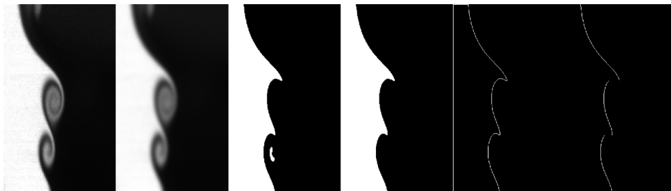
Figure 2. Step by step of obtaining the contour of the TNTI as T. Westerweel J. and Hofmann et al. (2002)
