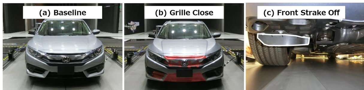
Fig. 2 Test vehicle configurations of (a) Baseline, (b) Grille Close and (c) Front Strake Off
