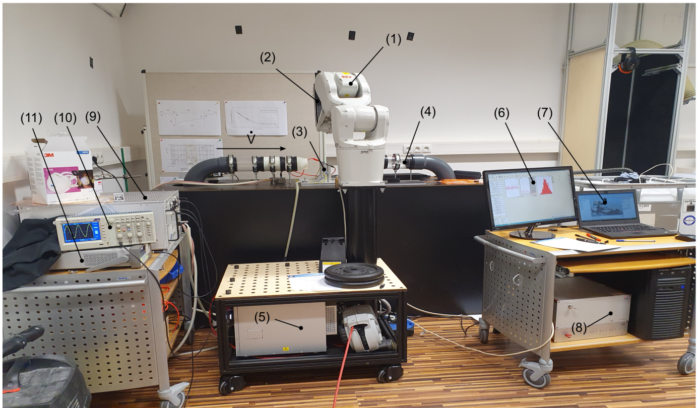
Figure 1. Experimental setup - LDA measurements: (1) ... robot ABB IRB 1200 7kg 0.7m, (2) ... LDA ILA fp50-shifted, (3) ... 30° inclined flat plate, (4) ... open wind channel, (5) ... robot control unit, (6) ... LDA measurement PC for post-processing, (7) ... Laptop with ABB RobotStudio®2021 to control the robot, (8) ... LDA raw signal processing including hardware filters, (9) ... high voltage power supply TRek 20/20C-HS, (10) ... scope Tektronik TDS 2002C, (11) ... function generator Agilent 33250A. The additional equipment used for smoke investigation is not shown. Fig. is taken from Berger et al. (2023).
