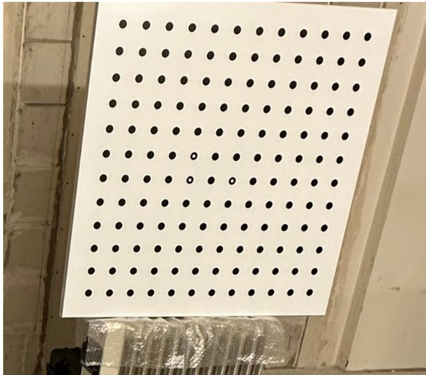
**Figure. 3** 2D-calibration plate for volumetric pinhole calibration. Five views at different locations and viewing angles have been recorded for bundle adjustment.
